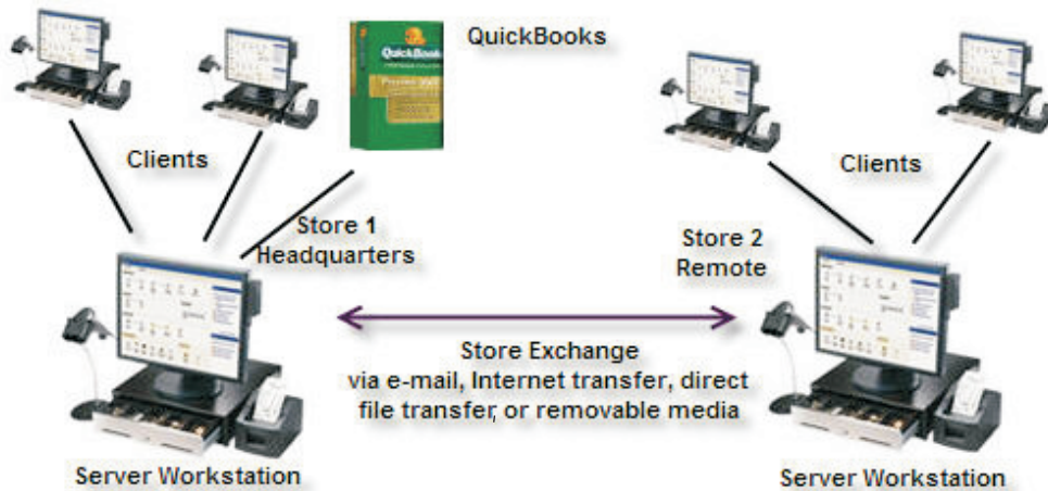
FIGURE 27-1 A typical two-store configuration
